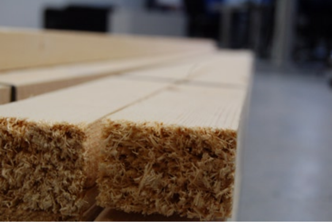
26-1: Laths from which the portal frame is made
